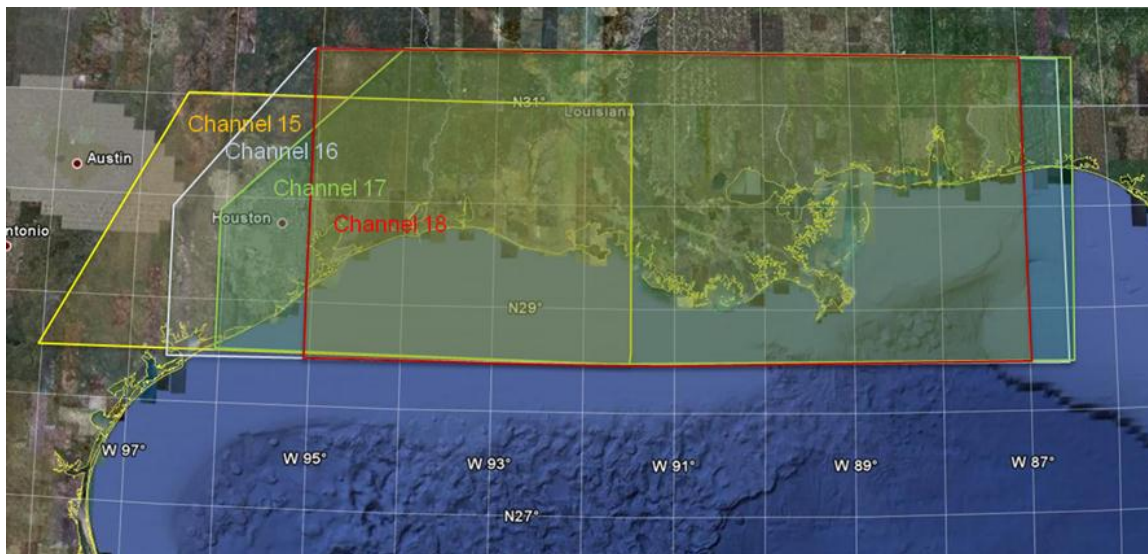
Figure 10 Map illustrating the geographic protection allotted to offshore radiotelephone services in the Gulf of Mexico
